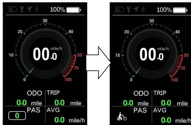
In the boost mode, the indicator is displayed dynamically. When the vehicle speed is less than 6km/h, release the "-" to stop the boost status. If no operation within 5s under static boost, it will be automatically jump to gear 0.
