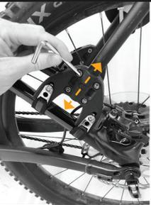
Depending on the size of your bike or seat, you can loosen the bolts shown above and slide the **spider rear rack** down to suit preferred height, and then tighten the bolts again.
