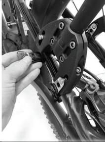
Start by unscrewing the bolts that loosen the 4 **straps** with allen key (see step 2 for bolt location). If you are using on a carbon frame we recommend a layer of standard bike tape or mastic tape on area of seat stays prior to install.
