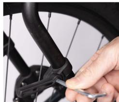
To install the lower pannier catch **anti-sway ingers**, loosen the **anti-sway finger** bolt so you can pull the clamp of the anti-sway finger apart enough to slide onto the **spider front rack**.
