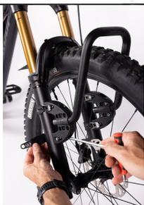
Position the **straps** on your front forks and connect the hole in the strap with the lug in the **feet**. Note the 2 holes in the straps. Choose the hole that best suits the thickness of your front forks. Once the **feet** are roughly in place, start tightening the **straps** using the allen key in the 4 bolts as shown in the next step.
