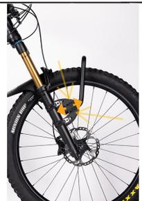
Depending on the size of your front forks/Bike, you can loosen the bolts shown above and slide the **spider front rack** into the attachment foot to suit preferred location, and then tighten the bolts again.
