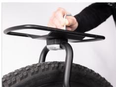
Installing the **Spider Pannier Receiver** is easy. The Spider Pannier Receiver mounts to the top of the **spider front rack**. Simply unscrew the 4 screws within the pannier receiver with a 5mm allen key, locate the male and female part of the pannier receiver on the **spider front rack**.
