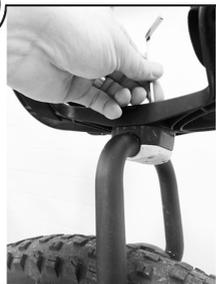
Installing the **Spider Rack Cradle** to the top or side of your Spider Front Rack is easy. Simply unscrew the 4 screws within the cradle with 5mm allen key, locate the male and female part of the cradle on the **spider front rack** tube and screw **cradle** back together.
